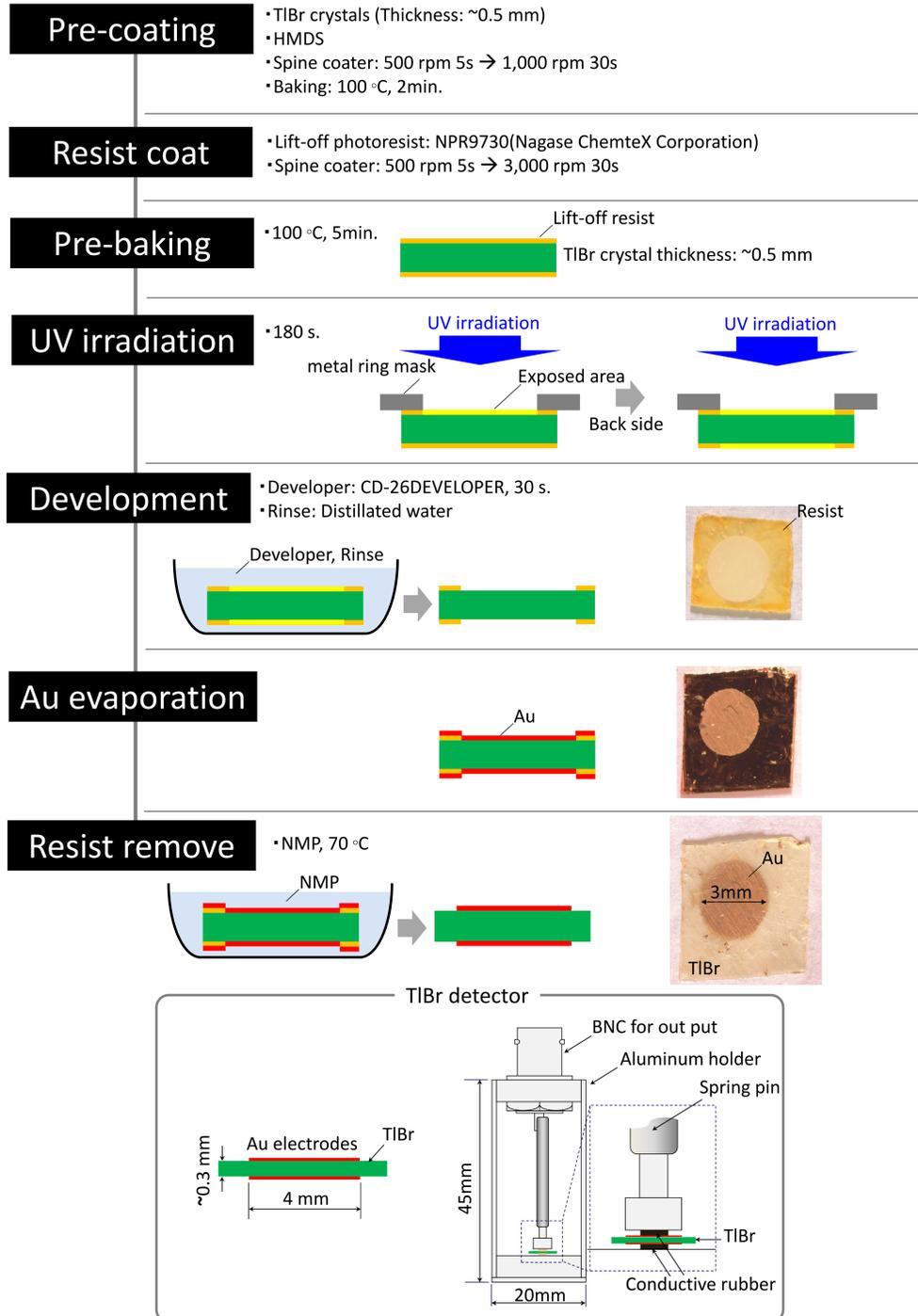
Fig. 6. Photoresist and electrode formation procedure for TlBr detector fabrication and schematic of TlBr detectors.
