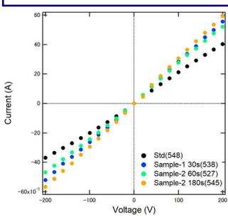
Fig. 7. I-V curves of TlBr detectors with Au electrodes formed by standard procedures and photoresist (irradiation time: 30, 60, 180 s).
