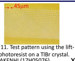
Fig. 11. Test pattern using the lift-off photoresist on a TlBr crystal.
