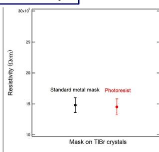
Fig. 8. Resistivity of TlBr detectors with Au electrodes formed by standard procedures and photoresist.
