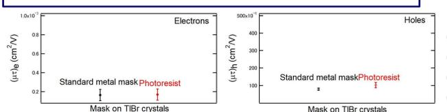
Fig. 9.  $\mu\tau$  products of TlBr detectors fabricated by the lift-off photoresist and a standard metal mask.
