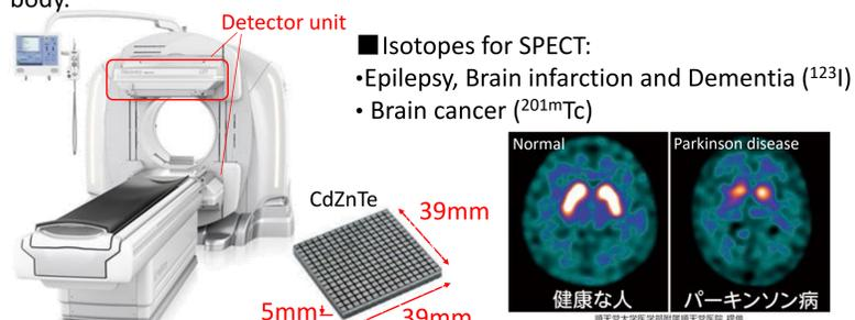
Fig. 1. SPECT and CdZnTe detector (GE Discovery NM/CT670CZT)
