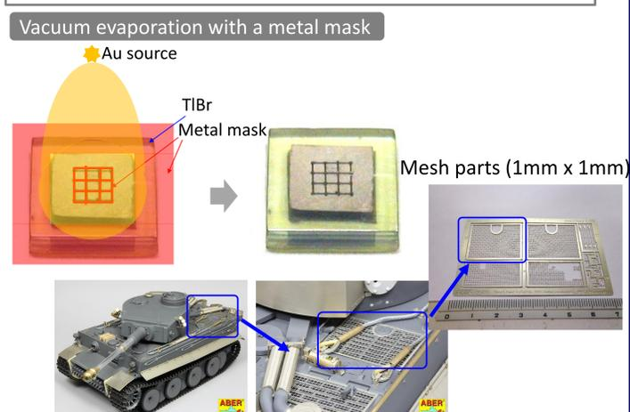
Fig. 5. Schematic of vacuum evaporation for forming pixel electrodes on TlBr detectors in our laboratory.
