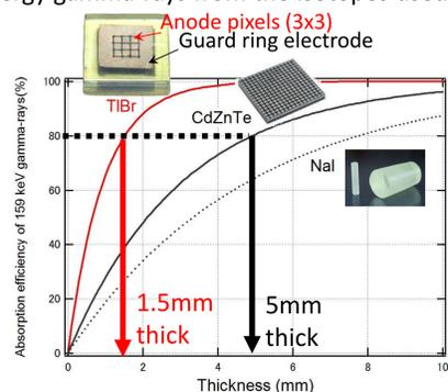
Fig. 4. Detection efficiency of TlBr, CdZnTe and NaI for gamma-rays (<sup>123</sup>I, 159 keV) used in SPECT diagnosis.
