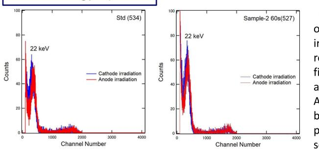
Fig. 10. <sup>109</sup>Cd energy spectra obtained from a TlBr detectors fabricated by the standard and photoresist procedure.
