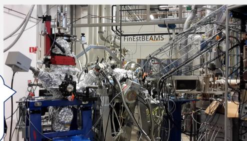
Luminescence excitation and emission spectra under excitation in the UV-VUV region were measured using the photoluminescence endstation of the FinEstBeAMS undulator beamline at the MAX IV synchrotron facility (Lund, Sweden).
