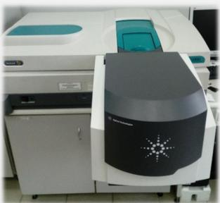
Absorption spectra were measured using an Agilent Technologies Cary-5000 spectrophotometer at 300 K and PerkinElmer Lambda 950 spectrophotometer in temperature region 80-500 K.
