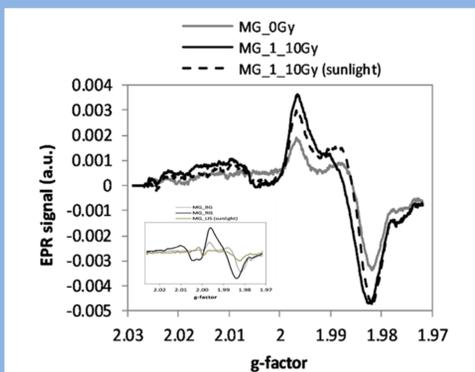
Figure 3. EPR spectra of MG samples: unirradiated (0 Gy), irradiated (10 Gy) and subsequently exposed for 5 min to sunlight). The inset presents the BG, RIS and LIS model spectra.
