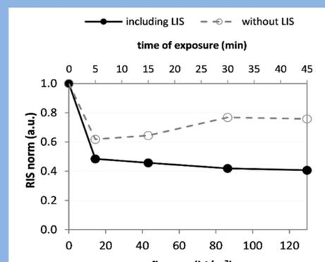
Figure 9. The dependence of on light fluence (CLEO UV lamp) and time of exposure in GG sample. The solid line represents data for the B-R decomposition (i.e. including LIS model spectrum) and the dashed line is for the B-R-L decomposition (i.e. neglecting the presence of the light-induced signal).
