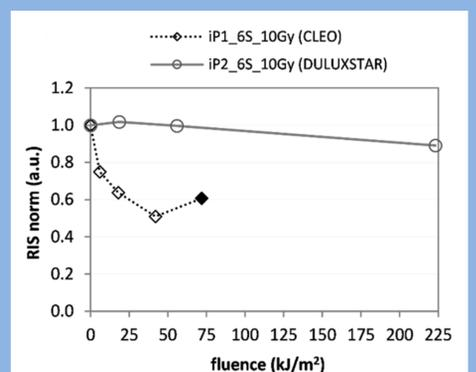
Figure 10. The dependence of RIS (B-R decomposition) on light fluence (CLEO UV lamp and DULUXSTAR) in samples from iPhone 6S. The DULUXSTAR lamp does not generate UV.
