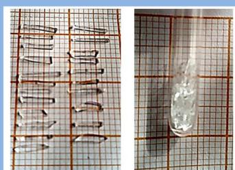
Figure 1. Crushed glass pieces and EPR sample tube filled with the sample on a graph paper.
