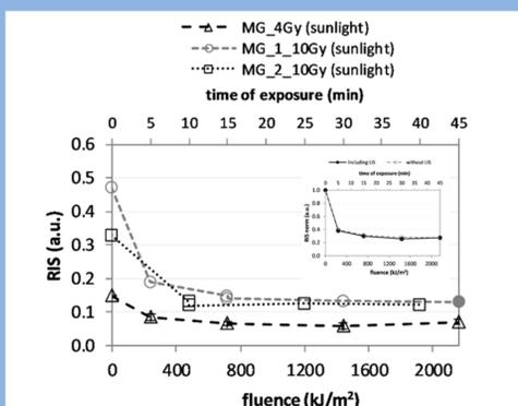
Figure 7. The dependence of RIS (B-R decomposition) on sunlight fluence (or time of exposure) in MG samples irradiated by X-rays to 4 Gy and 10 Gy and subsequently exposed to sunlight). The inset compares respective data for the MG\_1\_10 Gy sample for two decomposition procedures: using B-R and B-R-L model spectra sets).
