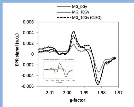
Figure 4. EPR spectra of MG samples: unirradiated (0 Gy), irradiated (10 Gy) and subsequently exposed for 45 min to CLEO UV lamp). The inset presents the BG, RIS and LIS model spectra.
