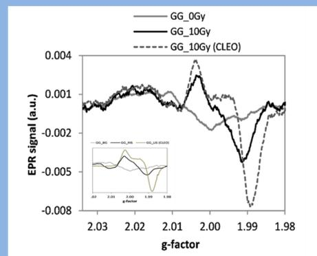
Figure 5. EPR spectra of GG samples: unirradiated (0 Gy), irradiated (10 Gy) and subsequently exposed for 45 min to CLEO UV lamp). The inset presents the BG, RIS and LIS model spectra.
