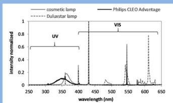
Figure 2. Emission spectra of the lamps used for illumination of the samples.
