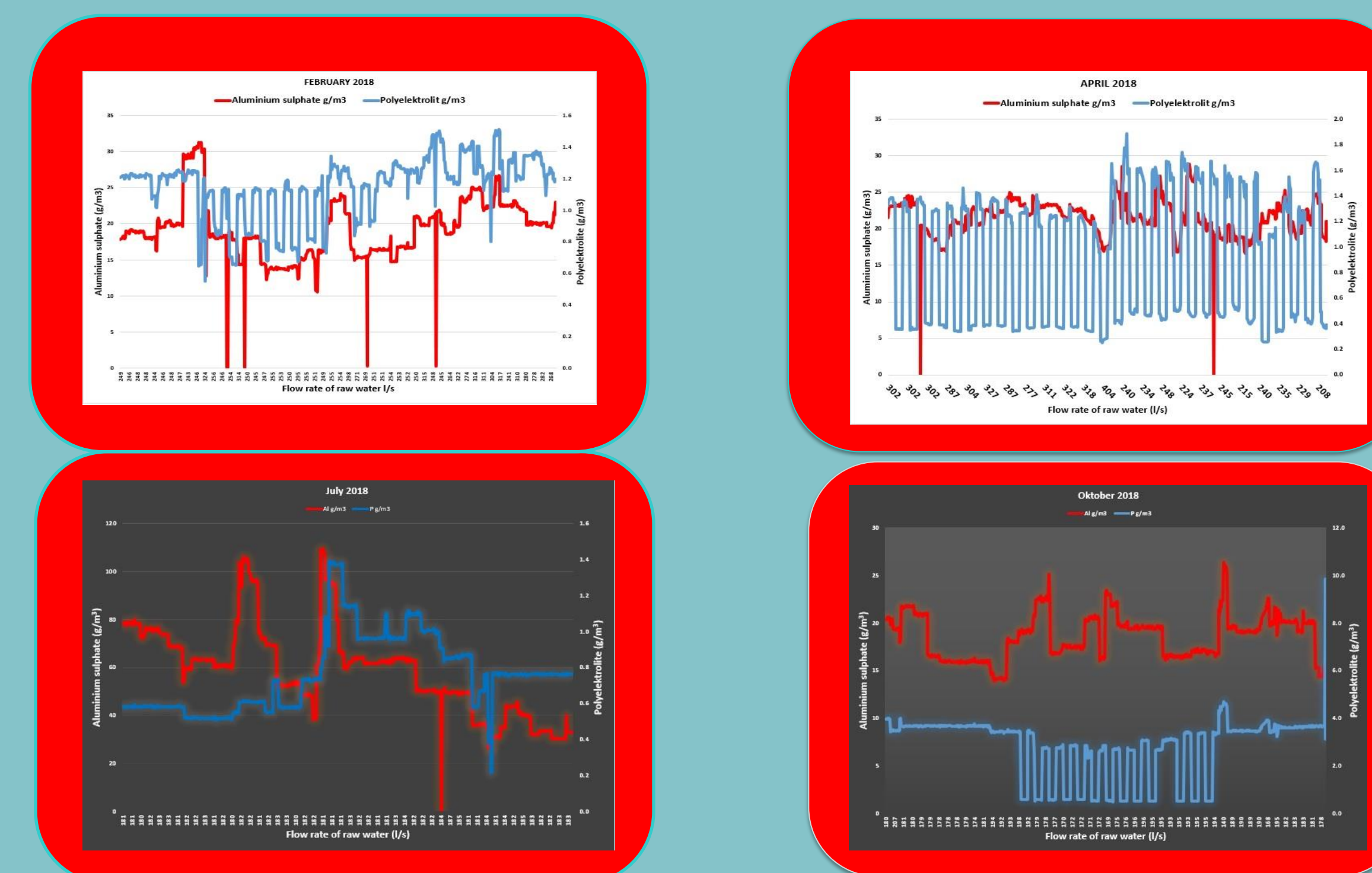
Figure 3 : The dependence of concentration of Al-sulphate and polyelectrolyte on the flow rate of Susicica water during representative months climate affected in 2018. year
